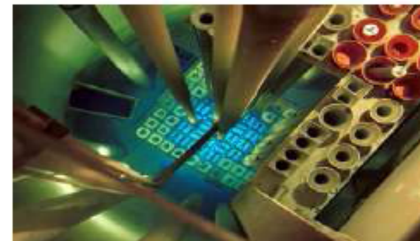
Cerenkov radiation in the reactor core in Budapest
