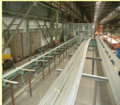
23 m long 9Cr-1Mo tubes under testing
