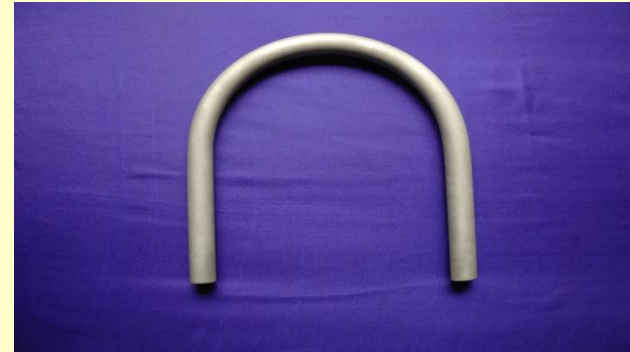
Glass Bead shot peened U bend Tube
