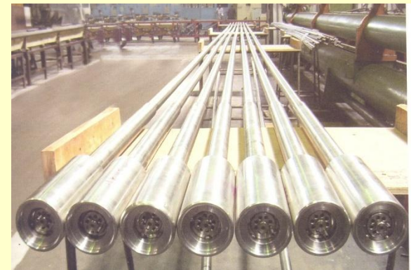
HORIZONTAL FLUX UNIT ASSEMBLY OF 13 METER LENGTH
