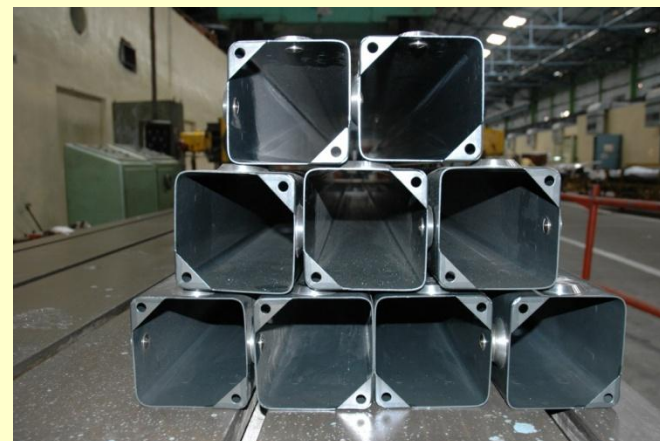
FINISHED SQUARE CHANNEL
